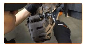
10 Remove the brake caliper.
