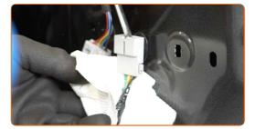
Attach the mirror adjuster connector to the door.
