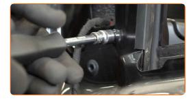
Treat the connector of the power mirror switch. Use dielectric grease.
