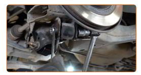
Unscrew the fastener connecting the stabilizer bar with the control arm. Use a combination spanner #16. Use a drive socket #18. Use a ratchet wrench.
