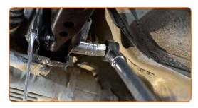
Tighten the fastener connecting the stabilizer bar with the control arm. Use a combination spanner #16. Use a drive socket #18. Use a torque wrench. Tighten it to 88 Nm torque.
