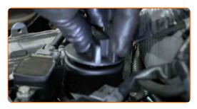
Tighten the oil filler cap.
