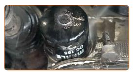
Unscrew the oil filter. Use the 65-14F socket. Use a ratchet wrench.
