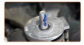
Install the serpentine belt tensioner pulley.
