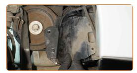
Screw the fixing bolts of the fuel filter bracket. Use a drive socket #13. Use a ratchet wrench.
