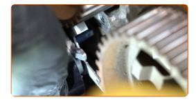
Install the new timing belt according to the factory marks.
