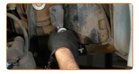
Remove the fuel filter fastening bracket.
