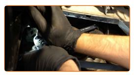
Screw in the subframe fasteners. Use a drive socket #18. Use a ratchet wrench.
