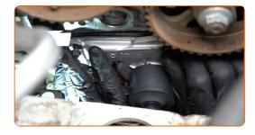
Tighten the water pump fasteners. Use a drive socket #8. Use a torque wrench. Tighten it to 12 Nm torque.
