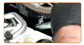
75 Treat the engine mount fasteners. Use a sealant.
