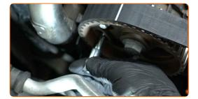
Remove the crankshaft gear locking tool.
