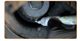
Loosen the fastener of the timing belt tensioner pulley. Use a combination spanner #13. Use HEX No.H6.
