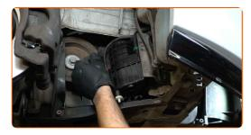
Pull aside the V-ribbed belt tensioner pulley. Use a combination spanner #16.
