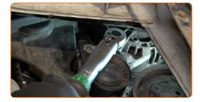
Unscrew the crankshaft pulley fastener. Use a drive socket #18. Use a ratchet wrench.
