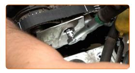
Install the upper timing cover. Make sure you hear a click indicating that it is locked in place.
