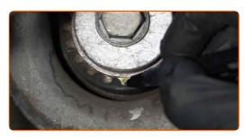
Install the camshaft gear locking tool according to the factory marks. Use an engine timing tool set.
