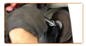
Remove the crankshaft pulley.
