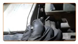
101 Install the fuel filter fastening bracket.
