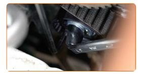
Remove the camshaft gear locking tool.
