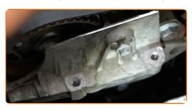
Tighten the engine mount fastening bolts. Use a drive socket #10. Use a torque wrench. Tighten it to 40 Nm torque.
