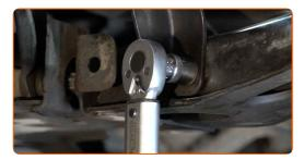
Tighten the subframe fastening. Use a drive socket #18. Use a torque wrench. Tighten it to 105 Nm torque.
