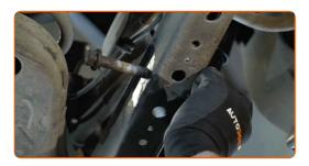
Remove the fastening bolt.
