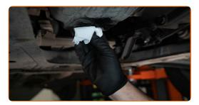
Screw in the new drainage plug and tighten it. Use a torque wrench. Tighten it to 34 nm torque.
