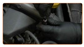
Detach the air intake hose clamp. Use combination pliers. Use a crowbar.
