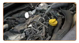
Detach the glow plug wiring connectors.
