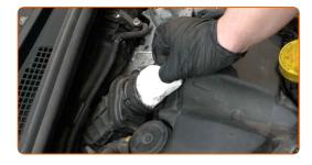
Install the air intake pipe and secure it.
