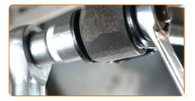
16 Tighten the fastener connecting the suspension arm to the car body. Use a combination spanner #17. Use a drive socket #17. Use a torque wrench. Tighten it to 98 Nm torque.
