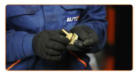
Install the lower cap onto the new fuel filter.
