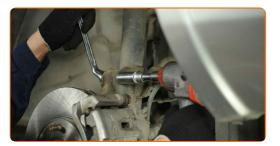
Remove the fastening bolts. Disconnect the steering knuckle from the shock absorber strut.
