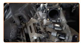
Tighten the intake manifold fasteners. Use a drive socket #10. Use a torque wrench. Tighten it to 27 nm torque.
