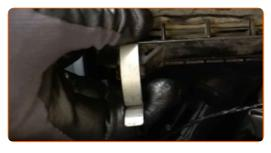
Slightly raise the cover of the air filter housing.
