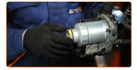
22 Install the new fuel filter together with its bracket.
