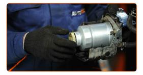
Install the new fuel filter together with its bracket.
