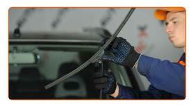
Remove the blade from the wiper arm.
