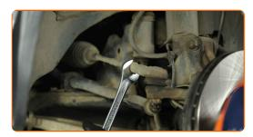
Remove the cotter pin fixing the tie rod end fastening. Use nippers.
