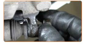
Remove the brake caliper.
