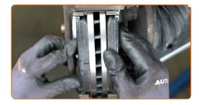
19 Install the brake caliper and fix it.
