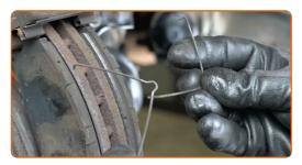
Remove the brake pads. Use a crowbar.
