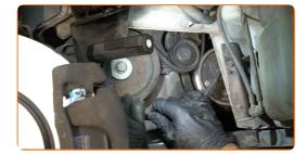
Return the tensioner pulley to its initial position. Use a combination spanner #16.
