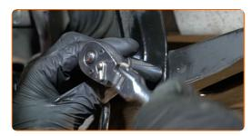
Unscrew the subframe fastening. Use a drive socket #18. Use a ratchet wrench.
