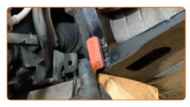
Unscrew the subframe reinforcement bracket fasteners. Use a drive socket #13. Use a ratchet wrench.
