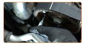
Remove the crankshaft gear locking tool.
