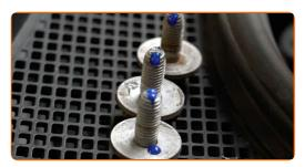
Tighten the upper fastener of the engine mount. Use a drive socket #16. Use a torque wrench. Tighten it to 76 Nm torque.
