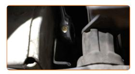
Remove the fuel filter fastening bracket.
