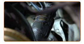
Attach the clamp of the lower coolant pipe. Use clic-R collar pliers.
