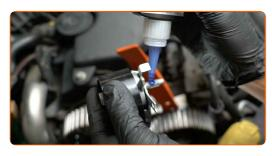
Install the timing belt tensioner pulley.
