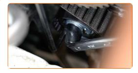
71 Remove the camshaft gear locking tool.
