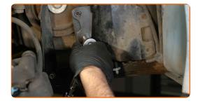
Remove the fuel filter fastening bracket.
