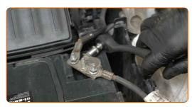
A Remove the battery terminals.
