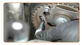
Make a mark on the camshaft gear.
