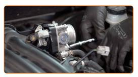
Attach the connector and the vacuum hose to the intake manifold near the throttle valve. Use round-nose pliers.
