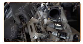
Tighten the intake manifold fasteners. Use a drive socket #10. Use a torque wrench. Tighten it to 27 nm torque.
