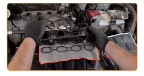
24 Install the intake manifold.
