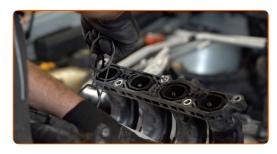
Install the new intake manifold gasket.
