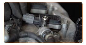
Unscrew the ignition coil bracket. Use a drive socket #10.
