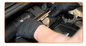
Reinstall the air filter cover. Fasten it.
