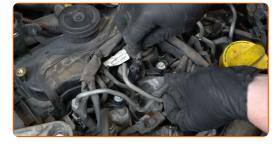
Unscrew the glow plugs. Use the spark plug socket #10. Use a ratchet wrench.
