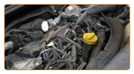
Detach the glow plug wiring connectors.
