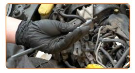
Treat the glow plugs. Use the injector & glow plug grease.
