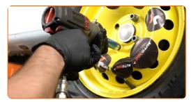
Lower the car and working in a cross order, tighten the wheel bolts. Use wheel impact socket #17. Use a torque wrench. Tighten it to 105 Nm torque.
