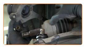
Disconnect the steering knuckle from the suspension strut.
