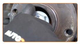
Screw in the fastener of the CV axle. Use a drive socket #30. Use a ratchet wrench.
