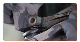
Disconnect the ball joint from the steering knuckle.
