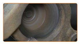
Install a new ABS sensor mounting ring.
