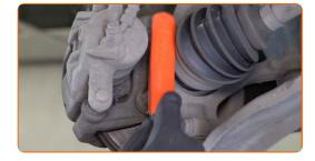
Unscrew the brake caliper bracket fasteners. Use a drive socket #17. Use a ratchet wrench.
