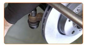
17 Tighten the tie rod end locknut. Use a combination spanner #17 (2 pieces). Use a torque wrench. Tighten it to 50 Nm torque.
