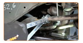
Unscrew the fastening nut connecting the tie rod end to the steering knuckle. Use a drive socket #14. Use a ratchet wrench.
