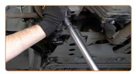
Tighten the rear fastener of the control arm. Use a combination spanner #18. Use a drive socket #18. Use a torque wrench. Tighten it to 127 Nm torque.
