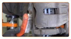
Treat the surface where the brake disc contacts the wheel rim. Use ceramic grease.
