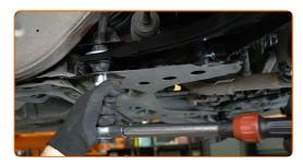
Tighten the ball joint fastener. Use a combination spanner #16. Use a drive socket #16. Use a torque wrench. Tighten it to 37 Nm torque.
