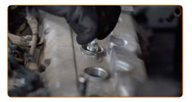
Screw new spark plugs and tighten them. Use the spark plug socket #16. Use a torque wrench. Tighten it to 19.6 nm torque.
