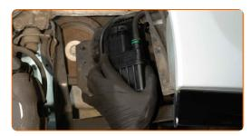
Screw the fixing bolts of the fuel filter bracket. Use a combination spanner #10.
