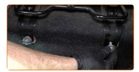
Screw in the front fasteners of the rear seat rails. Use a drive socket #17. Use a ratchet wrench.
