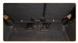
Remove the plastic covers of the rear seat rails. Use a clip removal tool.
