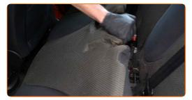
Remove the plastic covers of the rear seat rails. Use a clip removal tool.
