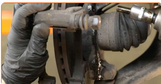
**17** Clean the brake disc fasteners. Use a wire brush. Use WD-40 spray.
