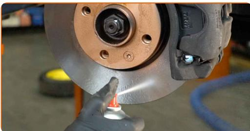
Replacement: brake discs – NISSAN Note (E11, NE11). Tip from AUTODOC:
