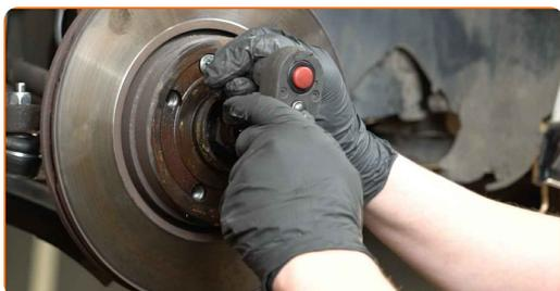
**19** Remove the brake disc.
