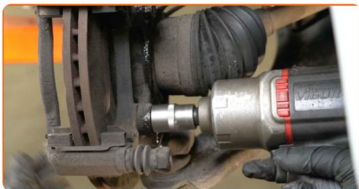
**16** Remove the caliper bracket.
