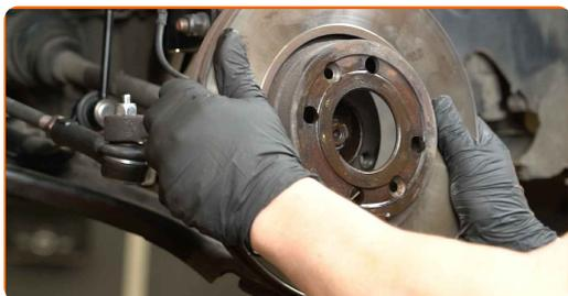
**20** Clean the hub. Use a wire brush. Treat the contacting surface. Use copper grease.
