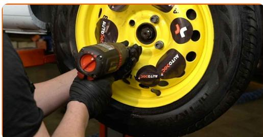
**35** Lower the car and working in a cross order, tighten the wheel bolts. Use wheel impact socket #17. Use a torque wrench. Tighten it to 105 Nm torque.
