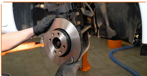
**22** Tighten the brake disc fastening. Use Torx T30. Use a torque wrench. Tighten it to 9 Nm torque.
