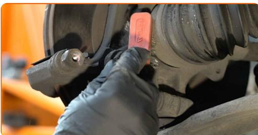
**15** Unscrew the caliper bracket fastening. Use a drive socket #18. Use a tap wrench.
