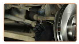
Install the cotter pin fixing the tie rod end fastening.
