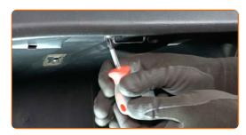
Remove the glove box cover retainers.
