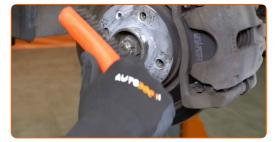
Unscrew the fastener connecting the drive shaft to the wheel hub. Use a drive socket #30. Use a tap wrench.
