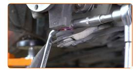
Tighten the lower fasteners connecting the shock strut to the steering knuckle. Use a combination spanner #17. Use a drive socket #18. Use a torque wrench. Tighten it to 116 Nm torque.
