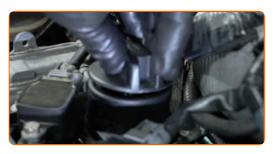
Tighten the oil filler cap.
