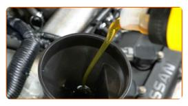
Replacement: engine oil and filter – NISSAN Micra IV Hatchback (K13KK).
