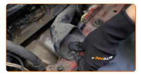
Remove the fender protection cover.
