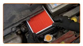
10 Install the air filter housing.
