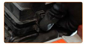
12 Install the air intake hose and secure it.
