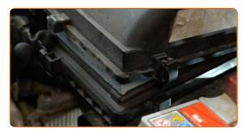
Lock the air filter housing retainers.
