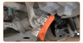
Unscrew the front fastener of the control arm. Use a drive socket #17. Use a ratchet wrench.
