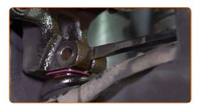
Disconnect the ball joint from the steering knuckle.
