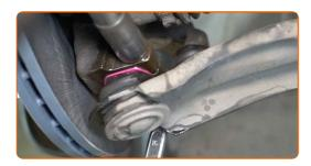
9 Remove the fastening bolt.
