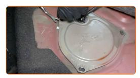
Clean the fuel pump module's mounting seat. Use all-purpose cleaning spray.
