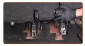
Release the retainers on the fuel pump module access cover. Use a Phillips screwdriver.
