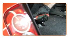
Reinstall the plastic covers of the rear seat rails.
