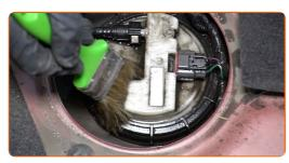
Detach the fuel pump module connector.
