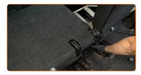
Move the rear seat rails to the side along with the backrest.
