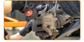
Clean the brake caliper fasteners. Use a wire brush. Use WD-40 spray.
