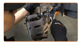
10 Remove the brake caliper.
