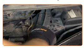
Screw in the fasteners of the cabin filter housing cover. Use a Phillips screwdriver.
