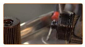
Install new O-rings (2 pieces) and a new oil filter to their mounting seats on the filter cover.
