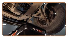
Unscrew the drain plug. Use square oil drain plug socket No.8
