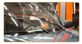
After installation check the wipers performance. The blades shouldn't intersect or bump against the windshield seal.
