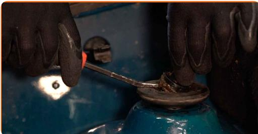
**4** Loosen the upper fastener of the shock strut mount. Use a combination spanner #21. Use HEX No.H6. Use a ratchet wrench.
