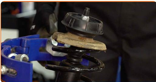
**29** Remove the assembled shock strut.
