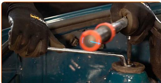
**40** Install the shock strut mount cap.
