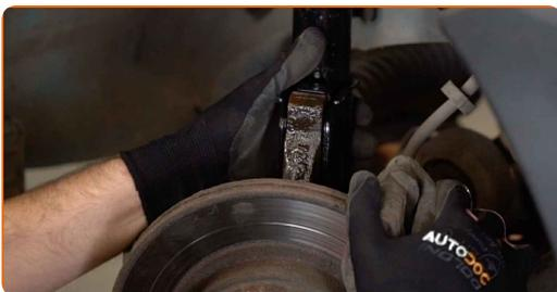
**34** Remove the support from under the steering knuckle.
