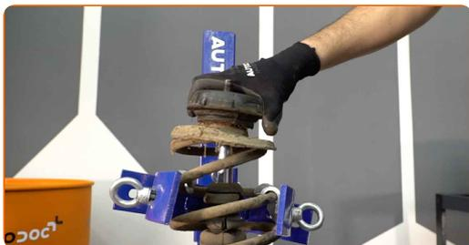
**20** Release the coil spring.
