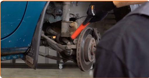
**11** Unscrew the lower fastener connecting the shock strut to the steering knuckle. Use a drive socket #21. Use a combination spanner #21. Use a tap wrench.
