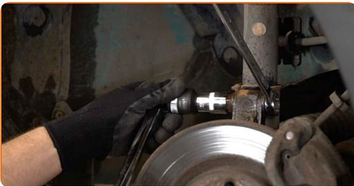
**12** Prop up the steering knuckle. Use a hydraulic transmission jack.
