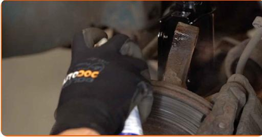
**32** Fix the shock absorber strut on the steering knuckle.
