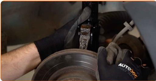
**33** Install and tighten new bolts of the steering knuckle. Use a drive socket #21. Use a combination spanner #21. Use a torque wrench. Tighten it to 140 Nm torque.
