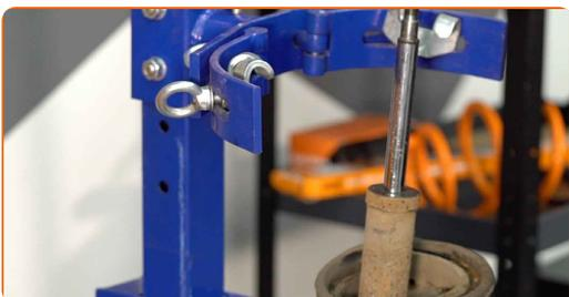
**23** Install the boot and a bump stop onto the shock absorber.
