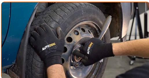
**38** Lower the car and working in a cross order, tighten the wheel bolts. Use wheel impact socket #19. Use a torque wrench. Tighten it to 110 Nm torque.
