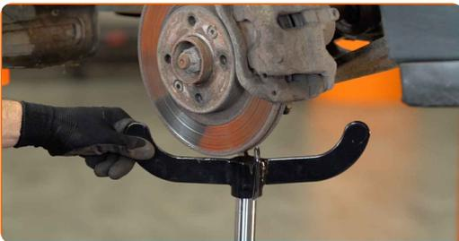
**13** Remove the fastening bolts (2 pieces). Use a hammer. Use a pin punch.
