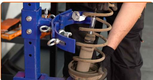
**22** Remove the shock absorber dust cap and the bump stop.
