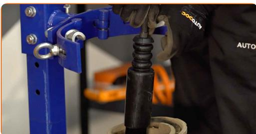
**24** Install the spring on the shock absorber.
