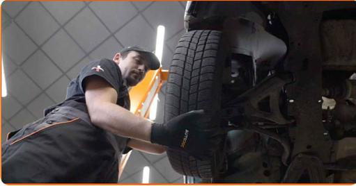
**10** Clean the shock strut fasteners. Use a wire brush. Use WD-40 spray.
