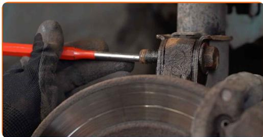
**14** Unscrew the upper fastening of the shock absorber strut. Use a drive socket #21.
