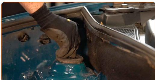
**41** Remove the fender protection cover.
