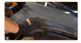
14 Install the fasteners of the wiper plastic cowl grille.
