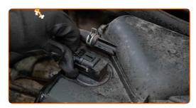
Insert the filter cartridge into the filter housing.
