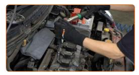
Treat the connectors of the ignition coils with an electrical contact cleaner spray.
