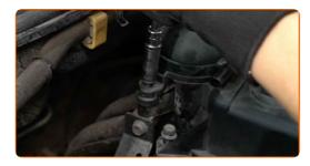
Attach the hoses to the engine cover and secure them with the clamps. Use long nose pliers.
