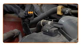
Loosen the clamps and detach the hoses from the engine cover. Use long nose pliers.
