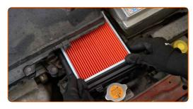
10 Install the air filter housing.
