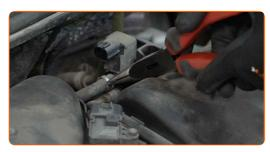
Unscrew the fasteners of the upper engine cover. Use a drive socket #10. Use a ratchet wrench.
