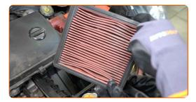
8 Move the air filter housing aside.
