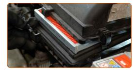
Lock the air filter housing retainers.
