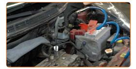
Unscrew the spark plugs. Use the spark plug socket #16. Use a ratchet wrench.
