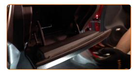
Unscrew the glove box fastening screws. Use a Phillips screwdriver.
