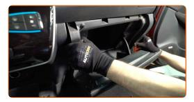
Screw the glove box fastening screws. Use a Phillips screwdriver.
