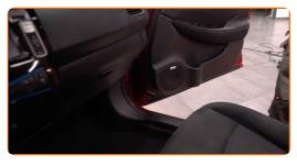
Remove the protective cover under the glove box.
