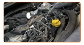
Detach the glow plug wiring connectors.
