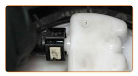
Attach the fuel pump module connector.
