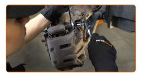
10 Remove the brake caliper.
