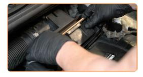
Reinstall the air filter cover. Fasten it.
