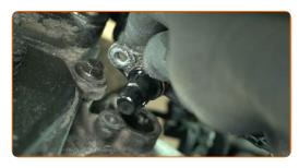
Plug the sensor mounting hole with a paper towel to prevent dust and dirt from getting in.
