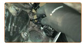
Install and screw in the fastening bolt. Use a 10 mm socket. Use a ratchet wrench.
