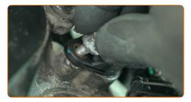
Tighten the fastener of the camshaft position sensor. Use a 10 mm socket. Use a torque wrench. Tightening torque: 10 N·m.
