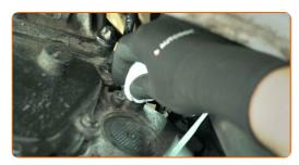
Clean the mounting seat of the camshaft position sensor. Use an all-purpose cleaning spray.
