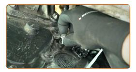
6 Remove the camshaft position sensor.
