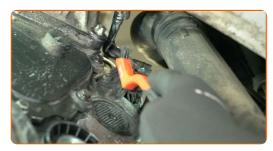
Detach the connector of the camshaft position sensor.
